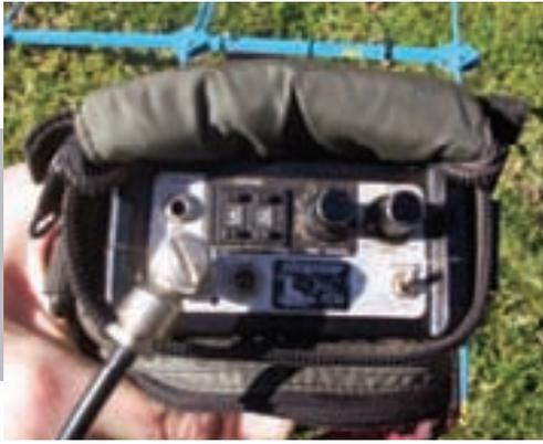
*Radio telemetry receiver with antenna in the background*
